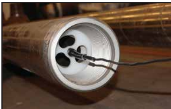
Cable saver (spider) as situated in the box of the pipe
