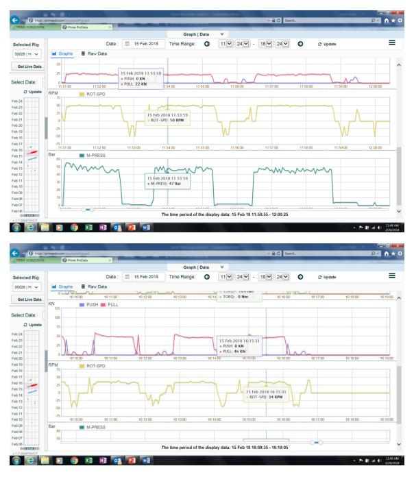
The graphs can be edited to show any paramater being measured by the Prodata system by selecting the EDIT LINE GRAPHS from the drop down menu in the top right hand corner (three horizontal bars).
