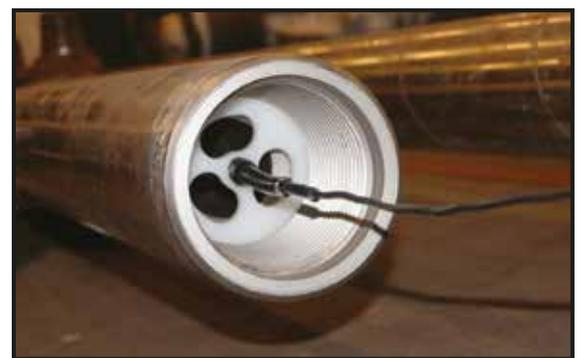
Cable saver (spider) as situated in the box of the pipe
