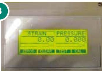
The Pull Head Driller Display Unit is a touch screen display. It receives information collected by the tail pipe data handler via radio frequency. The measured outputs are then displayed for the driller to see. The output allows the driller to initialize the system by calibrating the sensor output to 'zero' prior to beginning the pipe installation. It is also possible to change the pressure reading from Bar to PSI by applying the appropriate scale factor.
