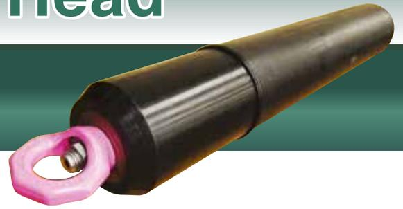
The Smart Pulling Head is an intelligent pulling head for high density polyethylene (HDPE) pipelines from 160 mm to 315 mm capable of measuring and transmitting pull force and down-hole mud pressure in real time.
