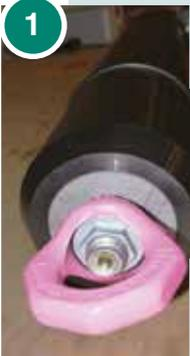
The Pulling Head is an industry standard Polyethylene pull head, modified specifically for the purpose of measuring down hole force and annular borehole pressures. The standard system can measure up to 30 tons of pull force and 400 bar of pressure.
