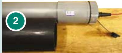
The tail pipe data handler is the electronic unit which is installed in the tail end of the product pipe. Its purpose is to receive the measured
