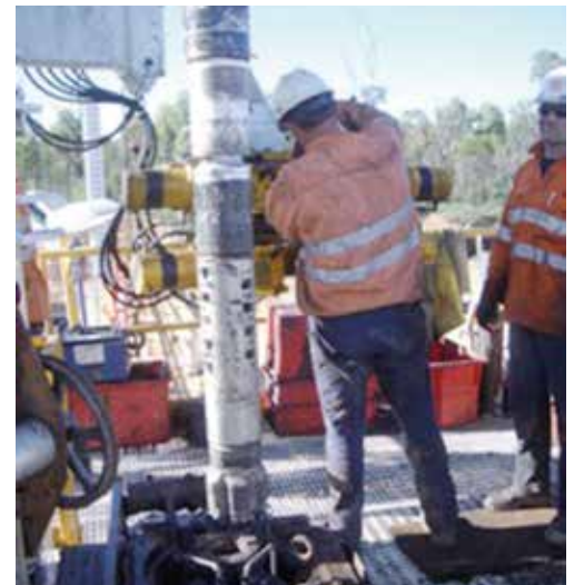
Figure 2-RMRS. The RMRS sub is located just behind the bit in this picture of a conventional, cantilever drilling rig. You can see the eight slots that contain the bar magnets. When the bit spins, the spinning magnets create the AC magnetic field.
