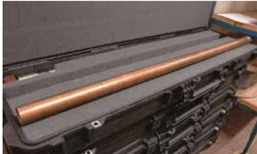
Shock mounted triaxial accelerometers and magnetometers, temperature sensor and digitising circuitry contained in 1.750 in. dia. x 55 in. long beryllium copper pressure barrel. Telemetry and power via single conductor wire line.
