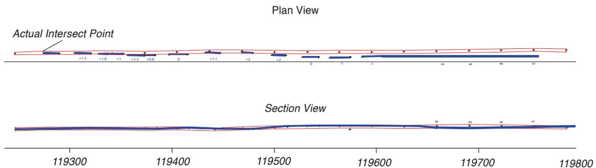
Michels Directional Drilling of Brownsville, WI, was contracted by Duke Energy to install a product line across a long stretch of water requiring an offshore crossing where casing was needed on each side of the crossing. The bore was drilled using conventional guidance techniques to a point about 3800 feet from entry. Difficult hole cleaning conditions prevailed requiring Michels to search for another solution.
