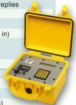
The RM Benchmark is a system that together with the 80+ rare earth magnets in its waterproof housing; includes the Acoustic Actuator and the Acoustic Deck Unit to remotely activate the submerged device.
